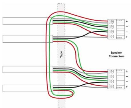
Connect the speaker cables to the VAE processor by inserting the two 4-pin connectors into the mating receptacles in the back of the processor. It does not matter which loudspeaker cable 4-pin terminal connects to which processor output as long as the color-coding is followed.
